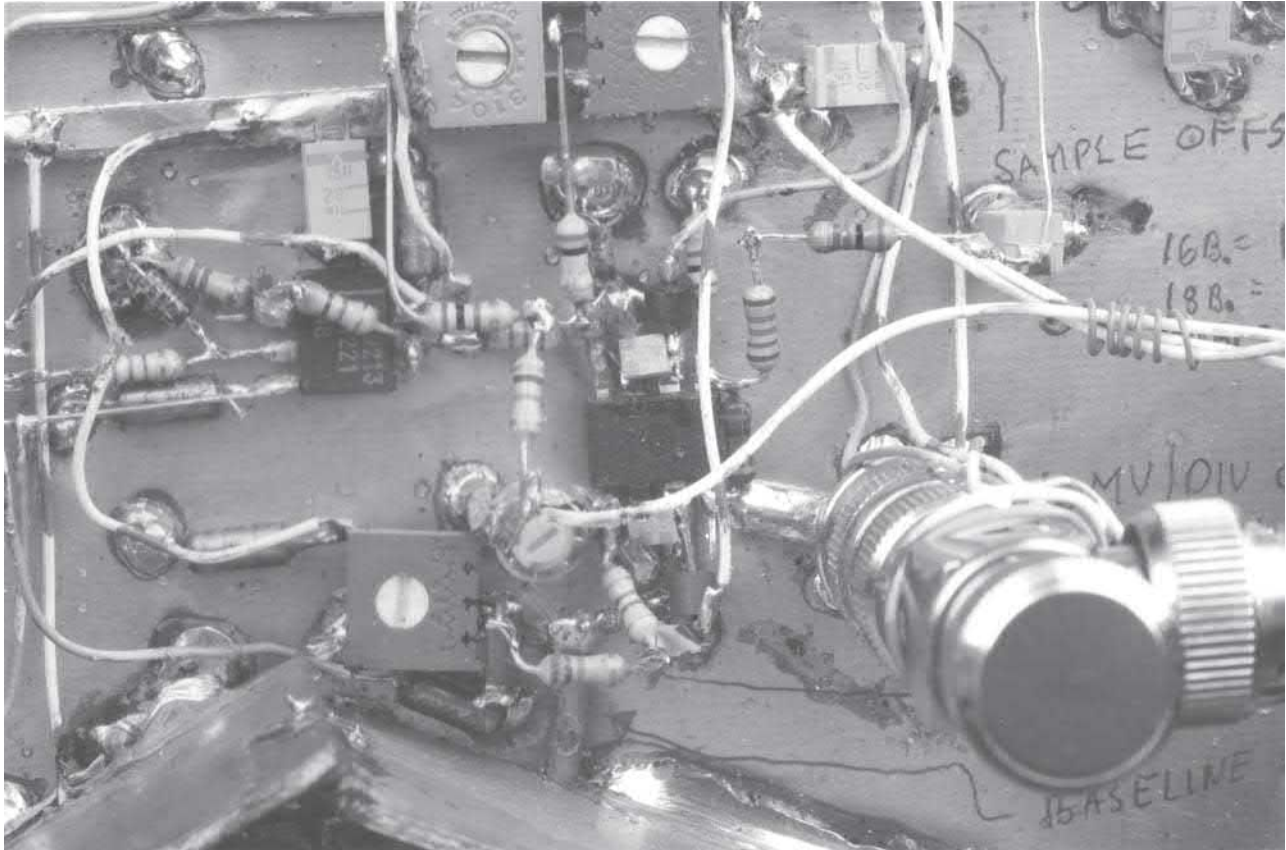
Figure G3 • LT1228 Sampling “Switch” (Photo Center) Is Mounted Upside Down, Permitting V^- Referred Die Backside To Shield Residual Radiative Coupling, Reducing Sampling Switch Drive Feedthrough. Switch Signal Channel Is Fed From Non-Saturating Amplifier (Photo Left). Sample Command From Shielded Digital Section (Lower) Arrives Via Coaxial Cable Tunneling Through Shield (Lower Center)
