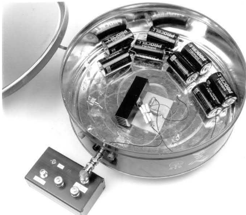
Figure 12.6b • Shielded Can with Cover Removed. LDO Under Test Occupies Center. D-Cells Provide Power, Eliminate Potential Ground Loop. BNC Fitting (Photo Lower Left) Connects Output to Filter Circuitry Test Box, Minimizing Triboelectric Based Errors
