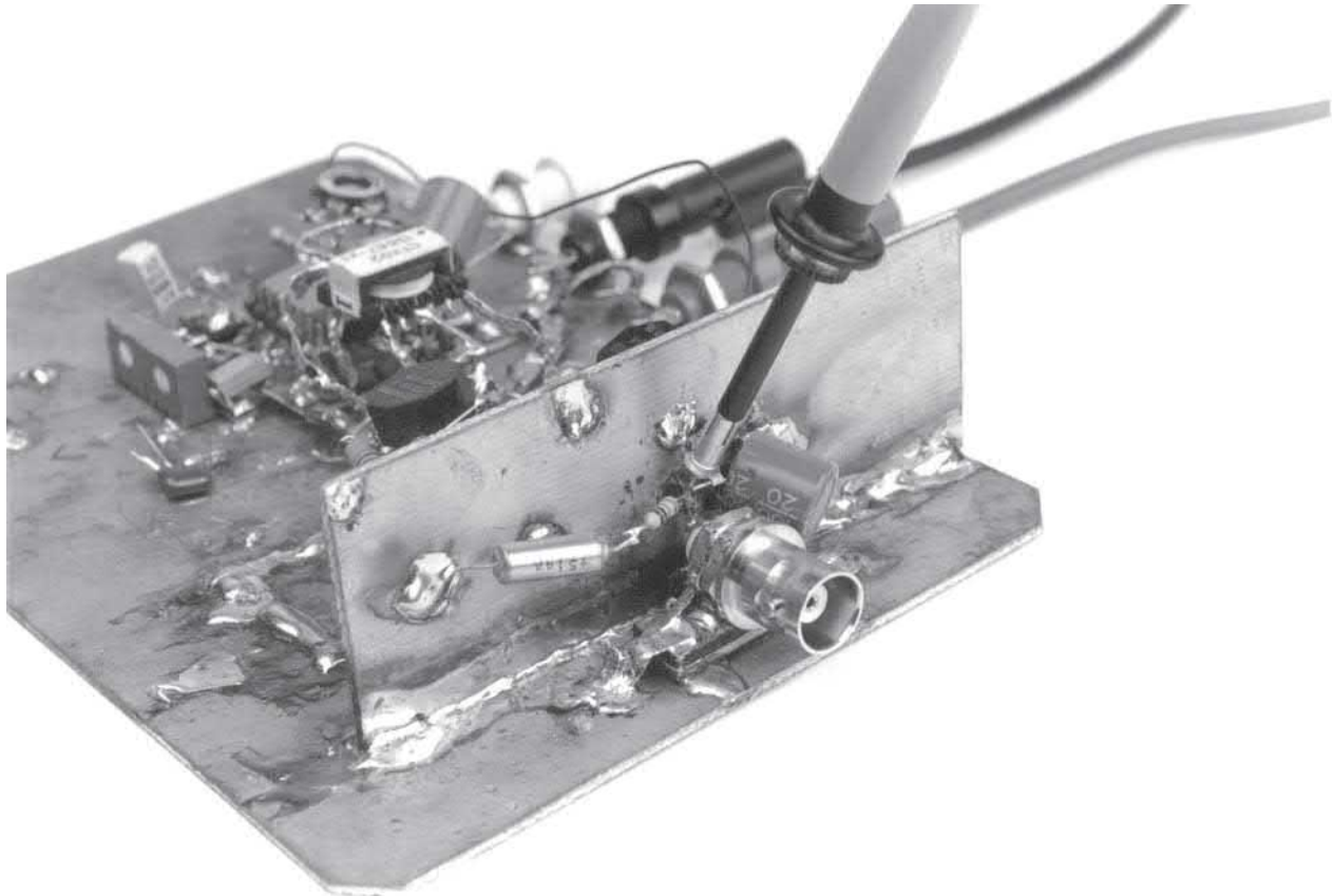
Figure C7 • Probe with Tip Grounding Attachment Approximates Coaxial Connection
