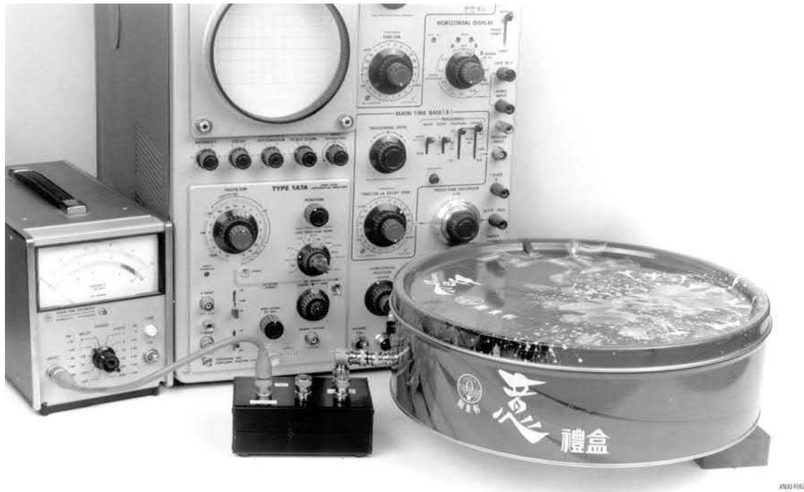
Figure 12.6a • LDO Noise Measurement Bench Setup. Shielded Can Contains Regulator; Noise Filter Circuitry Occupies Box at Photo Lower Center. Oscilloscope and RMS Voltmeter Are Not Simultaneously Connected, Precluding Ground Loop from Corrupting Measurement
