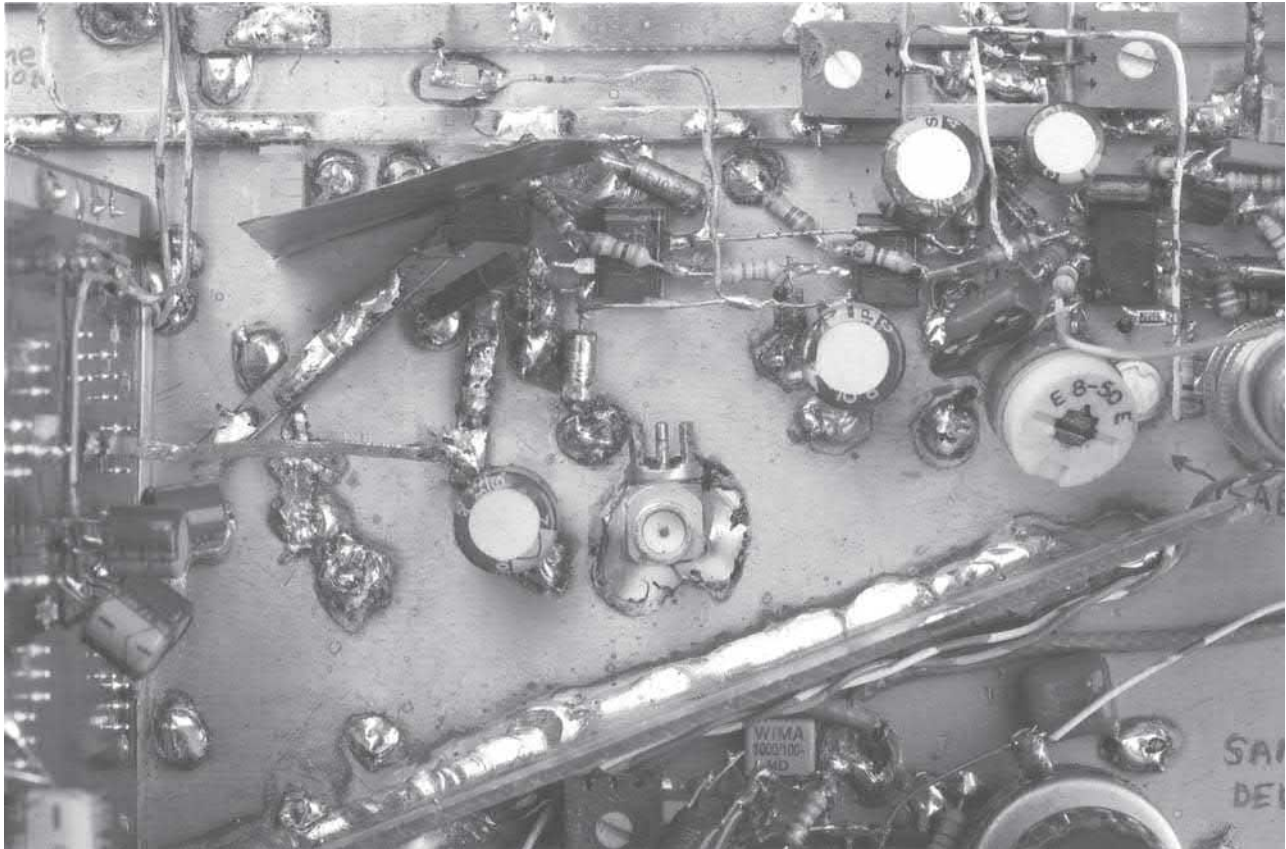
Figure G5 • Serially Interfaced Settling Time Breadboard Signal Path Detail. DAC Board is at Left. Precision Resistors Feed Summing Node and Non-Saturating Amplifier (Photo Upper Center). Shield Protects Summing Node from Input Pulse Originated Radiation. LT1228 Sampling “Switch” (Far Right) is Mounted Upside Down, Permitting V^- Referred Die Backside to Shield Radiative Coupling, Reducing Switch Drive Feedthrough. Switch Drive Level Shift-Current Source (Extreme Right Upper) Receives Sample Command Via Coaxial, Partially Visible at Lower Right. Large Vertical Shield Confines Sample Command Digital Section Radiation (Lower). SMA Connector (Center) Enables Test and Calibration Signal Connection
