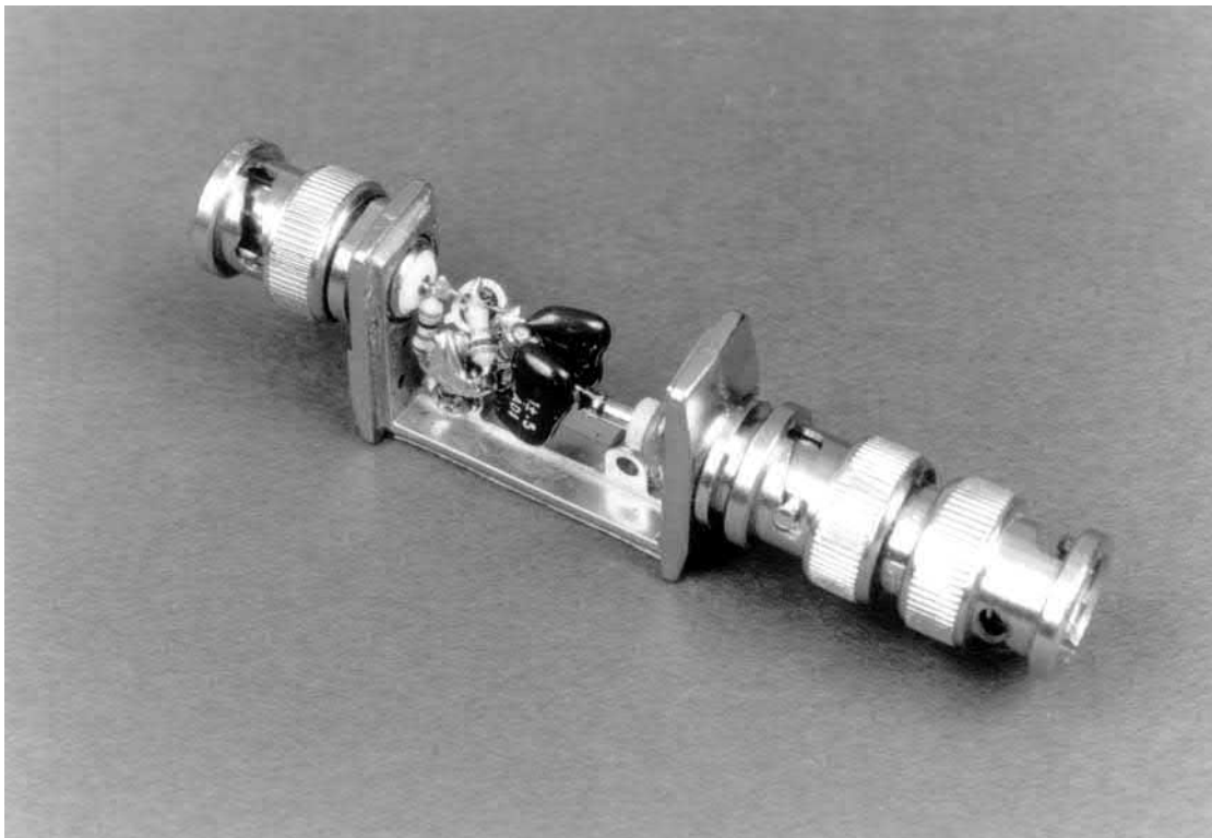
Figure B3 • Details of the Avalanche Pulse Generator's Head. 90VDC Enters at Lower Right BNC, Pulse Exits at Top Left BNC. Note Short Lead Lengths Associated with Output
