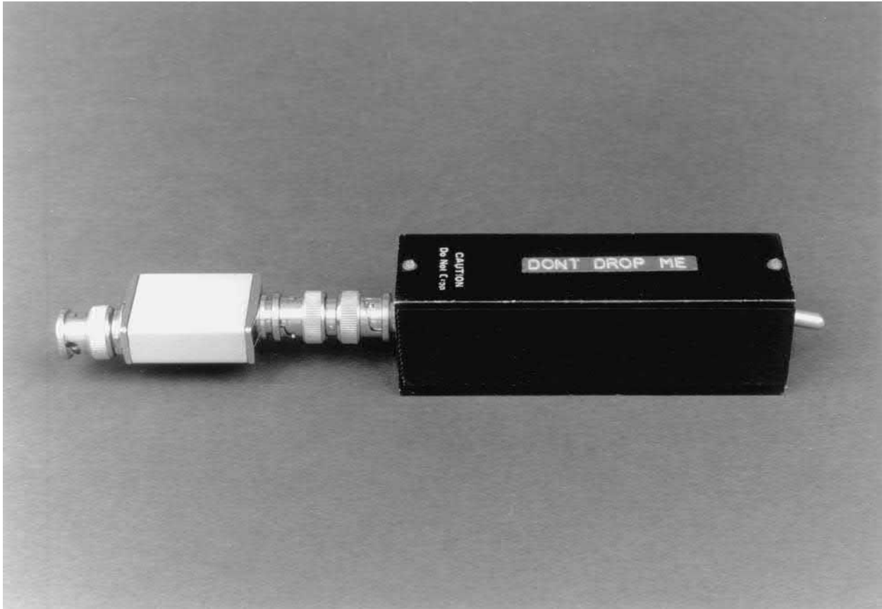
Figure B4 • The Packaged Avalanche Pulser. 1.5V-to-90V Converter Is in the Black Box. Avalanche Head Is at Left
