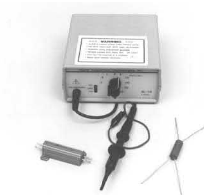
Figure C3 • Typical Current Shunts and an "Isolated" Probe
