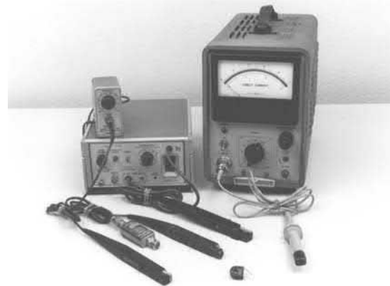
Figure C1 • Various Current Probe Types Provide Different Capabilities. Selection Criteria is Application Dependent
