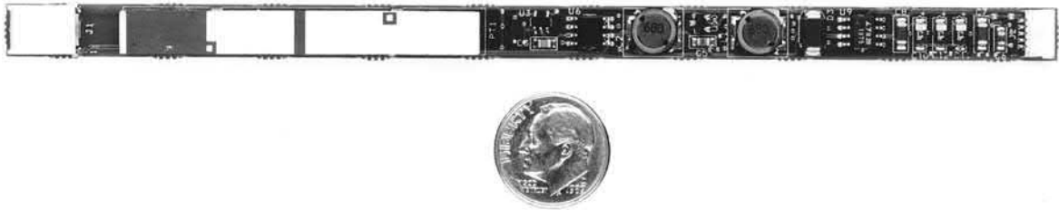
Figure 15.3 • Complete LCD Backlight Inverter Compared to Dime for Size. Piezoceramic Transformer (Photo Left) Permits Significantly Thinner Board Size
